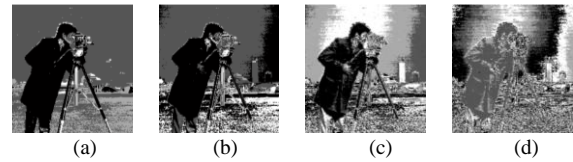
Figure 6. The retrieved results by superimposing different bit-plane, (a) bit-planes 7 and 8, (b) bit-planes 6 and 7, (c) bit-planes 5 and 6, (d) bit-planes 4 and 5.
