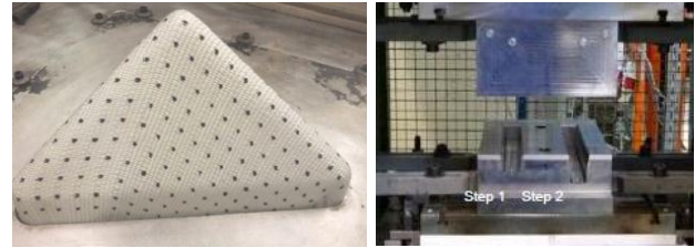
Figure 3. Tetrahedron pre-form for draping test (left) and thermoforming tools for profile pre-form (right)
